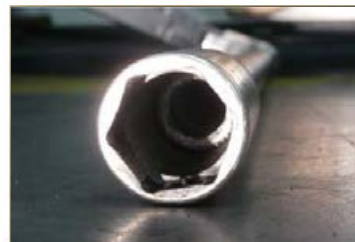
Socket with supports (not recommended)
